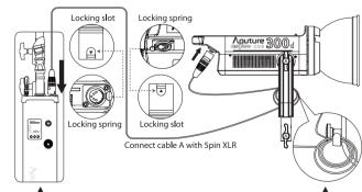
\* Hana the controller box on the tripod by buckle.
