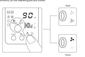
\* 1) Auto Mode: Fan speed is automatically adjusted according to internal temperature. ("Auto mode" is by default) \* 2) Force Mode: Fan operates at maximum speed. (Recommended for high temperature shoots)
