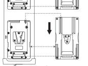
▲ V-Mount Battery \* Please use the output current 12A, capacity more than 190WH of the battery.
