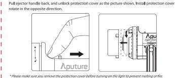
Please make sure you remove the protection cover before turning on the light to prevent melting or fire Put the cover back on the light after each use.
