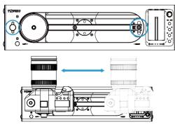
**2.6.2 Focus Shooting Mode:** Adjust the knob to th e upper left and lower right as shown below.
