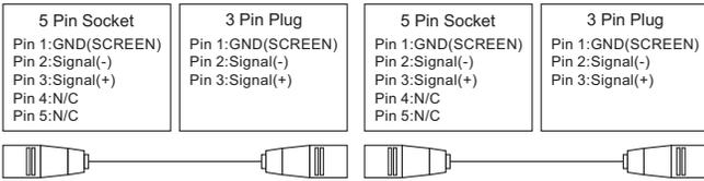
▲Notice: When using a 3-pin XLR plug, the Master / Slave Mode Control cannot achieve.
