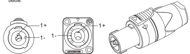
Pin1+: Connect the positive side of the power supply
