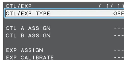
**2. Use the [VALUE] knob to specify “EXP” (expression pedal) as the device that’s connected to the CTL/EXP jack.**
