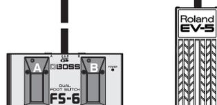
Connect an expression pedal (sold separately: EV-5, etc.) or footswitch (sold separately: BOSS FS-6, etc.). This is used when using your foot to control operations such as video switching.
