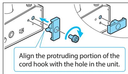
Align the protruding portion of the cord hook with the hole in the unit.
