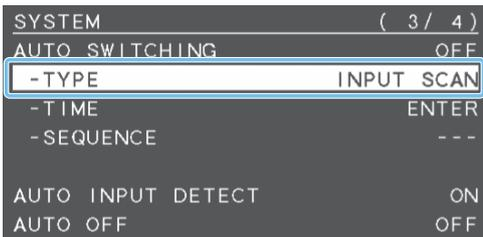
2. Use the [VALUE] knob to set "TYPE" to "INPUT SCAN," and then press the knob to confirm.
