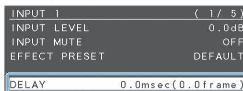
3. Use the [VALUE] knob to adjust the time by which the audio is delayed.
