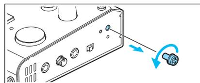
2. Using the screw that you removed in step 1, attach the cord hook as shown in the illustration.
