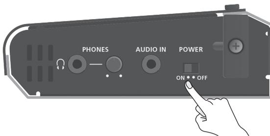
3. Turn on the power in the order of source devices → output devices.
