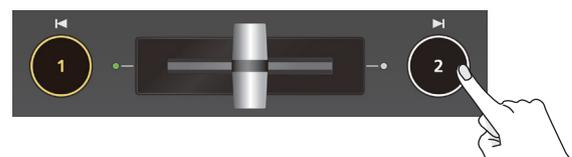
The composited result is output as the program. While it is output as the program, the [2] button and the KEY indicator are lit red. When you press the [2] button once again, the [2] button goes dark and the logo or image disappears.
