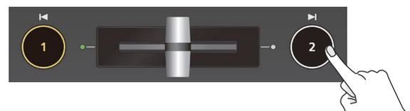
The composited result is output as the program. While it is output as the program, the [2] button and the KEY indicator are lit red. When you press the [2] button once again, the [2] button goes dark and the superimposed video disappears.
