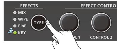
The KEY indicator is lit green, and the composition results is shown in the preview output video (standby video). You can check the key-composited video before you output to program.
