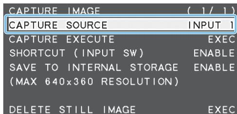
2. Use the [VALUE] knob to select either “INPUT 1” or “INPUT 2” according to the still image that you want to capture.
