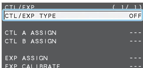
2. Use the [VALUE] knob to specify “CTL A & CTL B” (footswitch) as the device that’s connected to the CTL/EXP jack.
