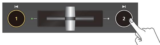
The inset screen is composited with the background video, and output as the program. The [2] button is lit red.
